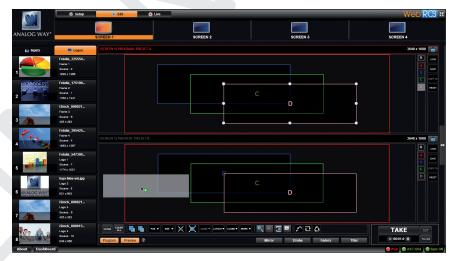
Your sources are now affected to layers. When a layer contains an input, it displays on the Web RCS an image into it or a live capture of the affected input. You can affect the inputs directly to any preset, even to the Program preset.
