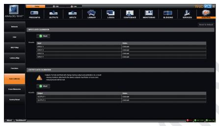
Choose Input or Output calibration and click and **START** button to launch the process.
