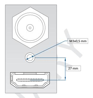
This hole is used by a TX10 screw when you receive the unit, if you wish to use an HDMI cable with a security fixing screw you can take this screw off and use your own in order to insure good fixing of your HDMI plug.
