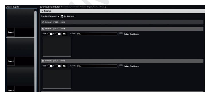
Drag and drop the available outputs into the desired screen. By default, your screens will mapped Output #1 = Screen #1, Output #2 = Screen #2 etc. You can change this order and put for example the Output #3 into the Screen #1
