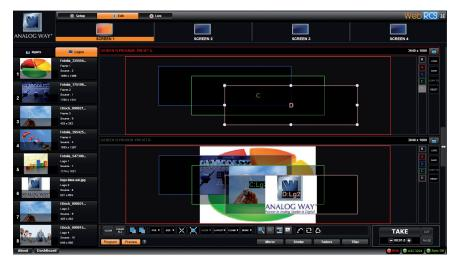
In this example, 4 inputs are affected to 4 layers into the Screen 1 Preview. The **TAKE** button on the bottom right side allows sending your configuration, made on the Preview screen, to the Program screen.
