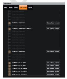
In this tab, you can define what is exactly the input format. The input format is automatically detected by the **Ascender 32** but you can change it or force it. The available formats are close to the current one, in terms of lines. This is only available for analog computer formats.
