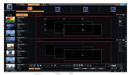
To display an input into one of the available layers A, B, C or D, simply drag and drop the input from the left to the layer on the chosen screen. Remember that a layer can be filled with an input but also with logos or frames.
