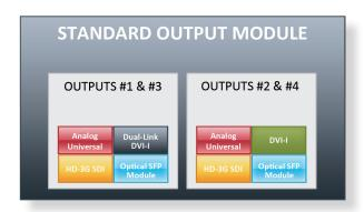
When using the standard output module for a dual-link DVI connection, connect the display to output #1. Output #2 will not be available when outputting a Dual-link DVI connection.
