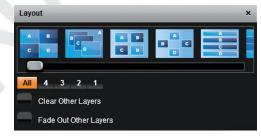
After having selected the layout, the changes are applied on the Preview screen. The size and position of all layers have changed. Of course you can still manage the new preset by positioning or resizing each layer thanks to the white circle around it.
