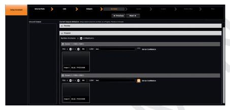
The confidence management allows a lot of settings on your confidence output. First of all you need to set up one of your output as a confidence output. To do that, please go under the preconfig menu, then "screens". Select one of your screens and enable the "SET AS CONFIDENCE" button. The confidence button is only available on Program screens.
